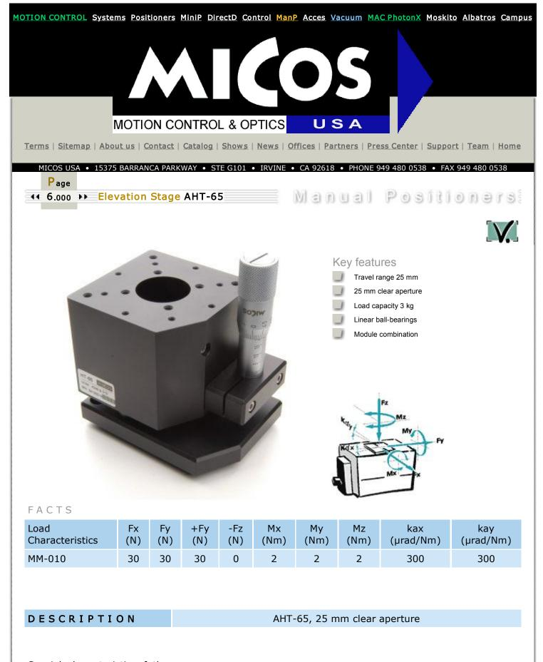
Special characteristic of the Elevation Stage **AHT-65** is its very compact structural shape. The module is suitable for the precise positioning of light construction parts. The translation is made with a Micrometer MM-010. Resolutions up to 10µm can be achieved.
